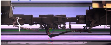
Automated detection of out-of-compliance air hoses
