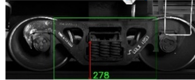
Automated measurement and detection of out-of-compliance truck geometry
