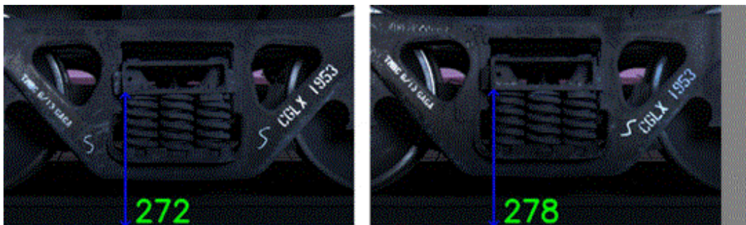
Truck Springs Geometry – Simultaneously Measured on Opposing Sides of Car at High Speed
