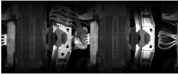
Ultra-High Definition Undercarriage Image at 46 MPH
