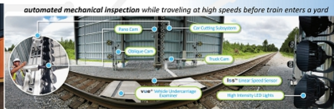
automated mechanical inspection while traveling at high speeds before train enters a yard
