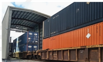
automated mechanical inspection while traveling at high speeds before train enters a yard
